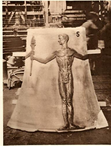
MADE IN PLASTER OF PARIS: A SECTION OF THE ACTUAL SHAPE OF THE BELL ON WHICH THE SCULPTOR HAS FORMED HIS MODEL.
