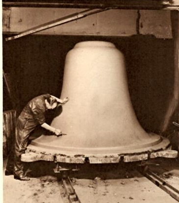
PREPARED FIRST AS IT TAKES THE LONGEST TO DRY OUT: THE CORE, WHICH IS SOLIDLY BUILT OF BRICKS AND LOAM SAND.
