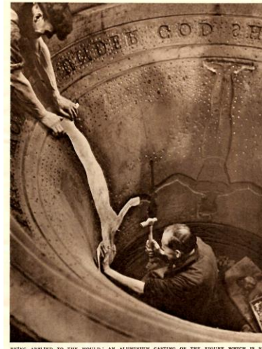
BEING APPLIED TO THE MOLD: AN ALUMINIUM CASTING OF THE FIGURE WHICH IS SKILFULLY PLACED IN POSITION BY THE MAN WHO APPLIED THE LETTERING.
