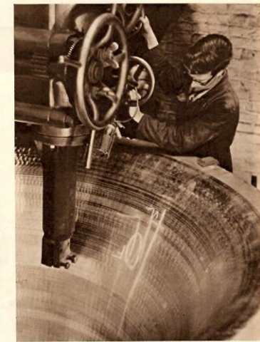
MACHINING THE INSIDE OF THE BELL IN PREPARATION FOR THE TUNING: AN OPERATOR CUTS THE METAL AWAY IN ACCORDANCE WITH THE CHALKED MARKS.
